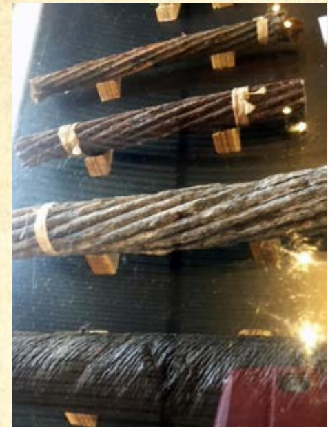
Examples of the Bass Strait cable which connected Tasmania to the world.
